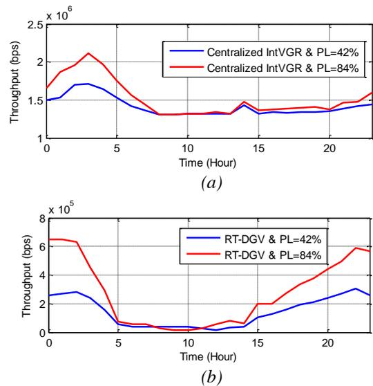
Figure 8: Throughput measured between the PEVs and the LVDN controller.
