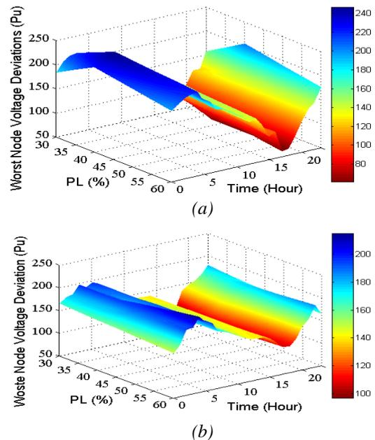
Figure 5: Voltage deviations in terms of different penetration levels (PLs) of the PEVs: a) Random charging scenario, b) RT-DVG scenario.
