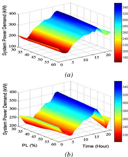
Figure 4: System power demand in terms of different penetration levels (PLs) of the PEVs: a) Random charging scenario, b) RT-DVG scenario.
