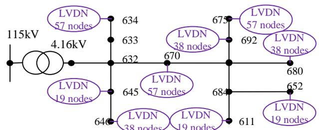
Figure 2: Single-line diagram of the power distribution network.
