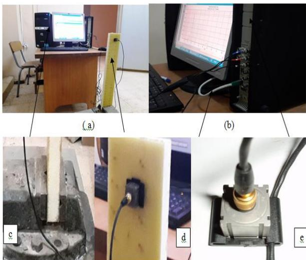
Fig. 2 Operating Mode : (a) Microcomputer and signal sensor (b) Mounting the sensors (c) Installation of the test piece (d) sticking the sensor to the free end ( e) Type 4506 tri-axial sensor.
