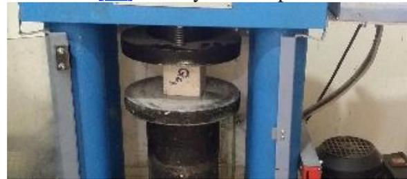
3000 kN capacity was used to evaluate the compressive strength on the identical cubic samples that were utilized in the previous two experiments. [Figure 5](#) shows the device used to measure compressive strength.
