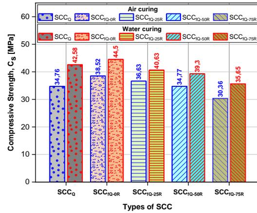
Figure 9. Results of compressive strength tests
