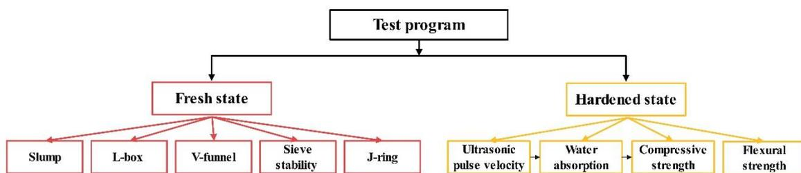
**Figure 2.** Test programs in fresh and hardened states
