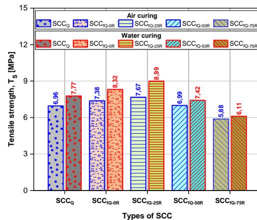
Figure 10. Results of tensile strength tests
