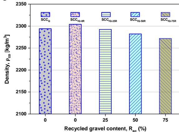
Figure 7. Effect of recycled gravel and steel fibers on density
