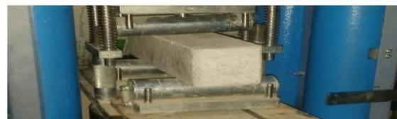
**Figure 6.** Device used to measure three-point bending strength.
