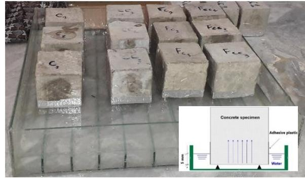
**Figure 4.** Water absorption test
