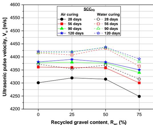
Figure 11. Results of the ultrasonic pulse velocity (UPV)
