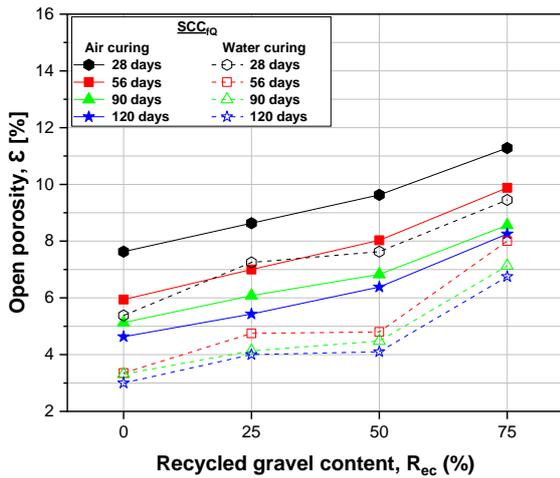
Figure 8. Effects of recycled gravel on the open porosity of SCC<sub>fQ</sub> in two curing regimes
