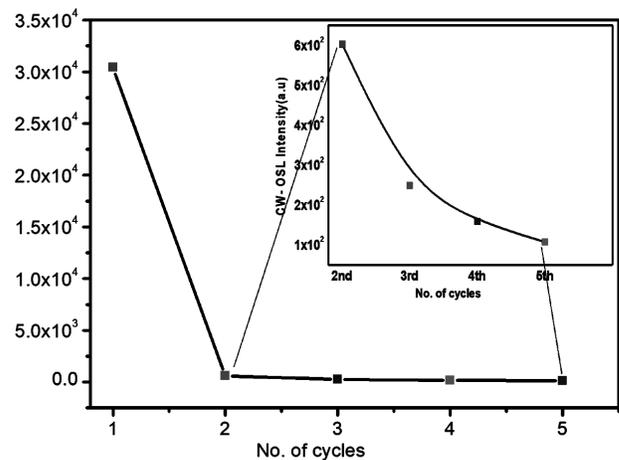
Fig. 8 — Cu<sup>2+</sup> doped NaLi<sub>2</sub>PO<sub>4</sub> Readouts many times irradiated with 10 Gy Co<sup>60</sup> Y-source. Shows OSL Intensity v/s no. of cycles. It is seen from Fig. 8 that during first readouts, more than 50% intensity was vanished. An expanded view of the successive readouts is shown in the inset of the figure.
