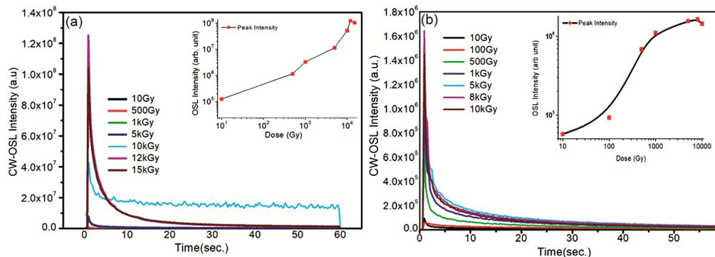
Fig. 6 — (a) OSL Dose response curve (ranging from 10Gy-15kGy) of  $\text{NaLi}_2\text{PO}_4:\text{Cu}^{2+}$  stimulated by the blue LED ( $80\text{mW},470\text{nm}$ ) before irradiation the 0.1mol% phosphor material annealed at 1073K for 1.0 h, (b) OSL Dose response curve (ranging from 10Gy-8kGy) of  $\text{NaLi}_2\text{PO}_4:\text{Cu}^+$  stimulated by using blue LED ( $470\text{nm}, 80\text{mW}$ ). The phosphor was annealed at 873K for 1h before irradiation with 0.08 mol%.
