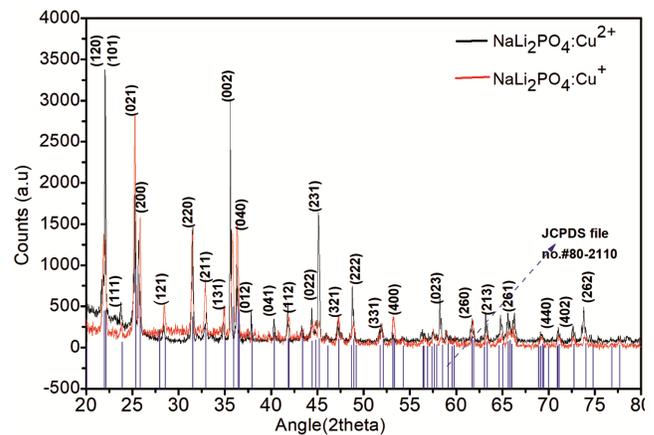
Fig. 1 — XRD form of the  $\text{NaLi}_2\text{PO}_4$  phosphors (our material). The data available in the literature" JCPDS File# 80-2110" is also given for comparison.
