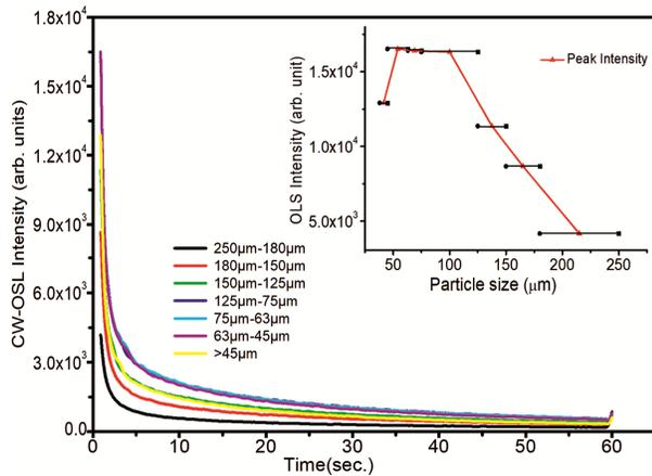
Fig. 5 — Particle size effect on  $\text{NaLi}_2\text{PO}_4:\text{Cu}^{2+}$  irradiated at  $\gamma$ -ray  $\text{Co}^{60}$  source.
