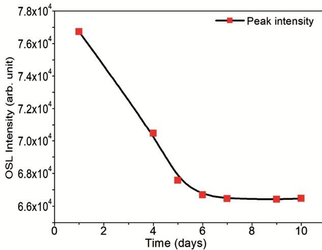
Fig. 9 — Typical CW-OSL decay curves of  $\text{NaLi}_2\text{PO}_4:\text{Cu}^{2+}$  taken 1.0hr after irradiation and storing in dark at room temperature (300K). Fading was taken starting from the same day up to 10 days.
