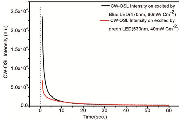
Fig. 4 — Effect of the stimulation source on the CW-OSL decay curves of  $\text{NaLi}_2\text{PO}_4:\text{Cu}^{2+}$  stimulation by Blue LED ( $80\text{mWcm}^{-2}$ ) and green LED ( $80\text{mWcm}^{-2}$ ). The material was irradiated at 10Gy of  $\gamma$ -ray  $\text{Co}^{60}$  source.
