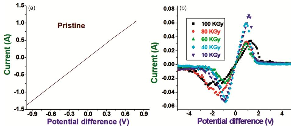
Fig. 3 (a-b) — I-V characteristics of (a) pristine, and (b) gamma ray exposed zinc 1D nanostructures.
