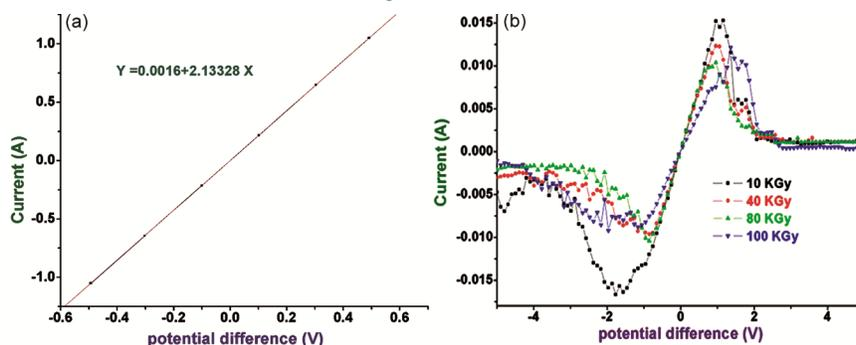
Fig. 2 (a-b) — I-V graphs of (a) pre-exposed, and (b) radiation exposed silver 1D nanostructures.
