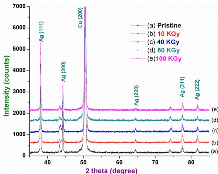
Fig. 4 — X-ray spectrum of (a) pre & post gamma irradiated silver 1D nanostructures with different doses of, (b) 10 KGy, (c) 40 KGy, (d) 80 KGy, and (e) 100 KGy.
