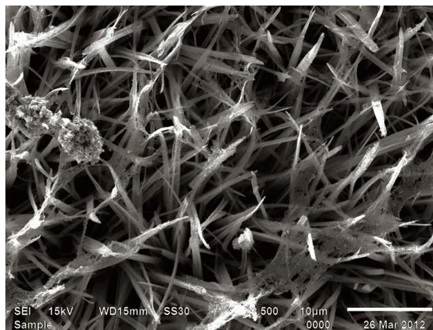
Fig. 1 — SEM image of silver 1D nanostructures.
