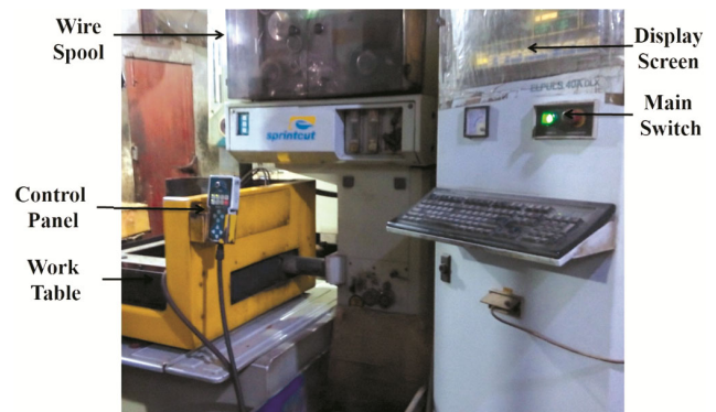
Fig. 2 — Experimental Setup — photographic view of CNC Wire – cut EDM
