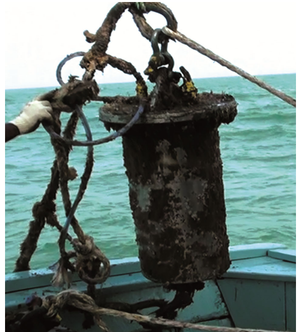
Fig. 10 — The retrieved Subsea pressure housing with SS316 L deployed off Goa.
