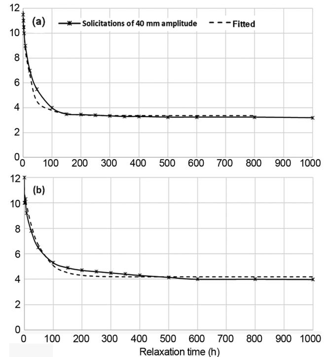
Fig. 3 — Non-linear fitting relaxation curve of knitted fabric following 6000 fatigues cycles (a) cyclic deformations of amplitude 40 mm and (b) cyclic deformations of amplitude 60 mm.
