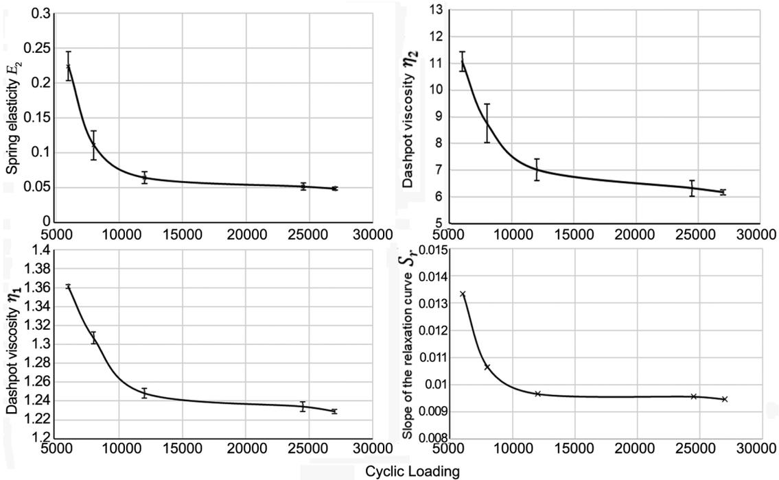
Fig. 7 — Evolution of Burger's model parameters according to number of fatigue cycles
