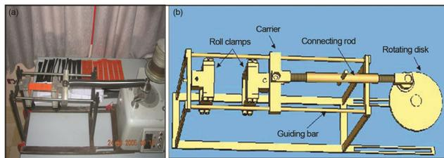
Fig. 1 —Fatigue device for fabric: (a) photography and (b) schematic diagram
