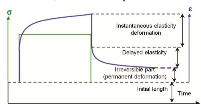
Fig. 5 — Burger's model deformations during a creep-recovery test.
