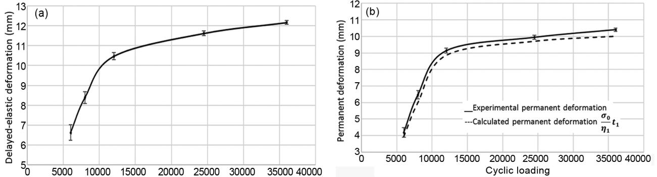
Fig. 6 — Evolution of delayed-elastic (a) and permanent deformation (b) according to the number of fatigue cycles
