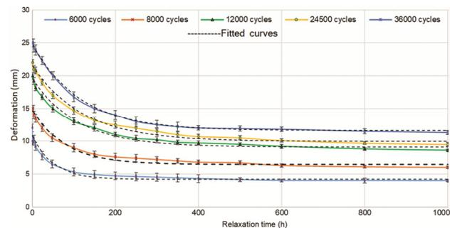
Fig. 4 — Evolution of fitted and calculated curves relaxation of knitted fabric after fatigue test
