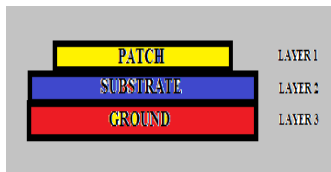
Figure1. Three layer structure of microstrip patch antenna
