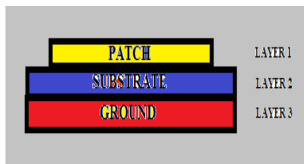
Figure 1. Three layer structure of microstrip patch antenna
