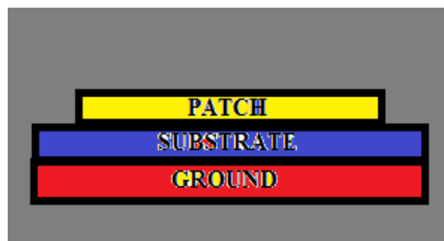
Figure 1. Three layer structure of microstrip patch antenna
