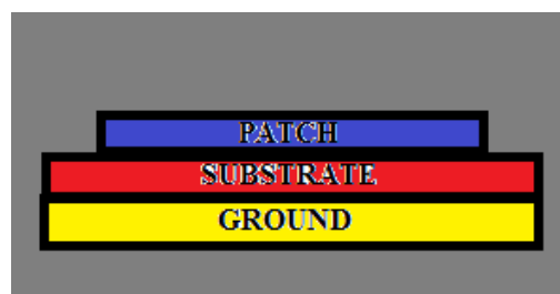
Figure 1. Three layer structure of microstrip patch antenna
