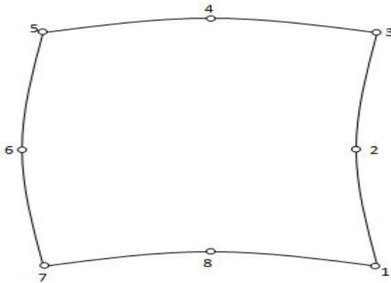
Fig. 1. 8-node isoparametric element
