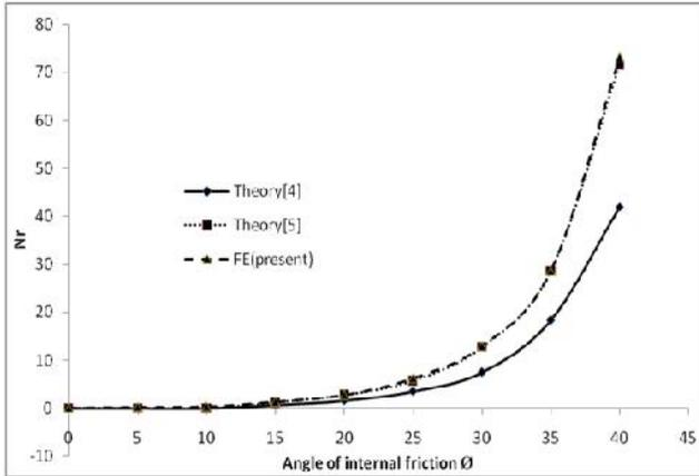
Fig. 6.  $N_\gamma$  for Rough footing with  $C=0$
