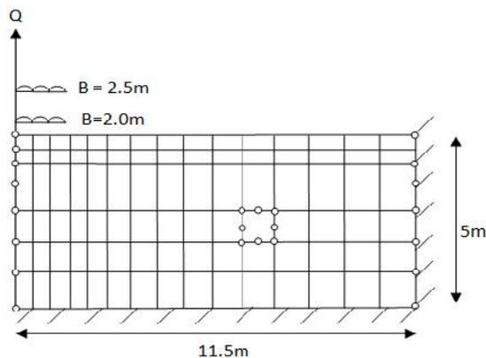
Fig.2. Finite Elements mesh for bearing capacity
