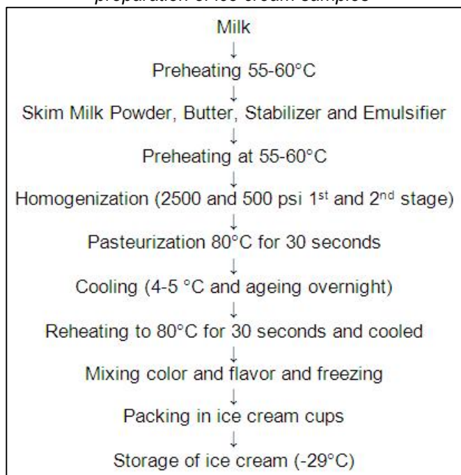
Fig.1. Process flow chart for the preparation of ice cream samples
