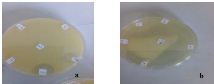
Figure 4. ZnS zone of inhibition against S. aureus (a) and E. coli (b)
