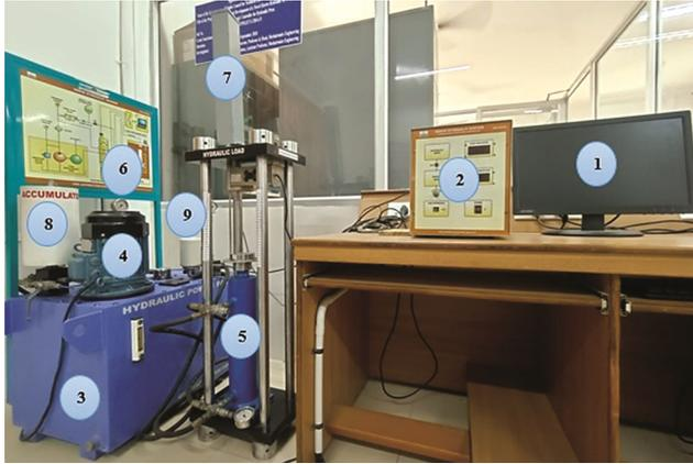
Fig. 2 — Photography of EHSS: 1-Personal computer (PC), 2-DAQ, 3-Hydraulic power pack, 4-Three phase fixed displacement pump, 5-Double-acting hydraulic cylinder, 6-Pressure gauge, 7-LVDT, 8-Accumulator, 9-Servo spool valve
