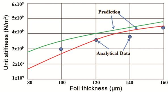
Fig. 5 — The unit stiffness verification by testing the thickness of its foil
