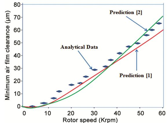
Fig. 4 — Confirmation of minimum air film thickness with the prediction
