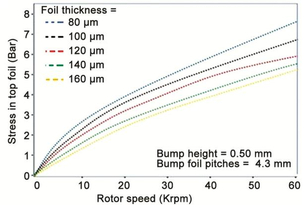
Fig. 3 — Deviation of stress in top foil against rotor speed
