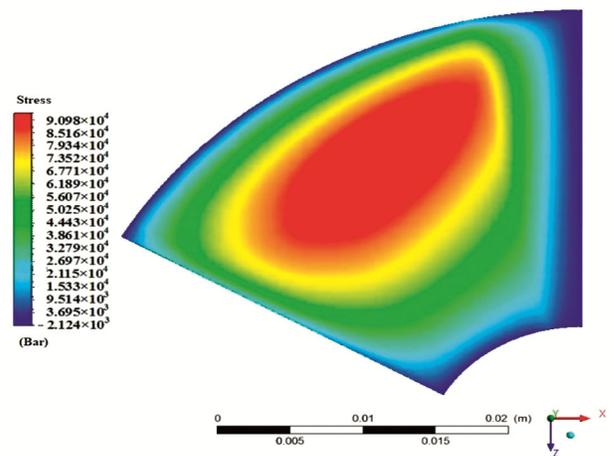
Fig. 1 — Stress analysis of top foil
