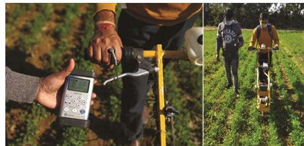
Fig. 11 — Instrument set-up for vibration measurement in the field
