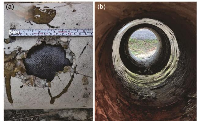
Fig. 12 — Retrofitting trials of damaged portion of the sewer pipe
