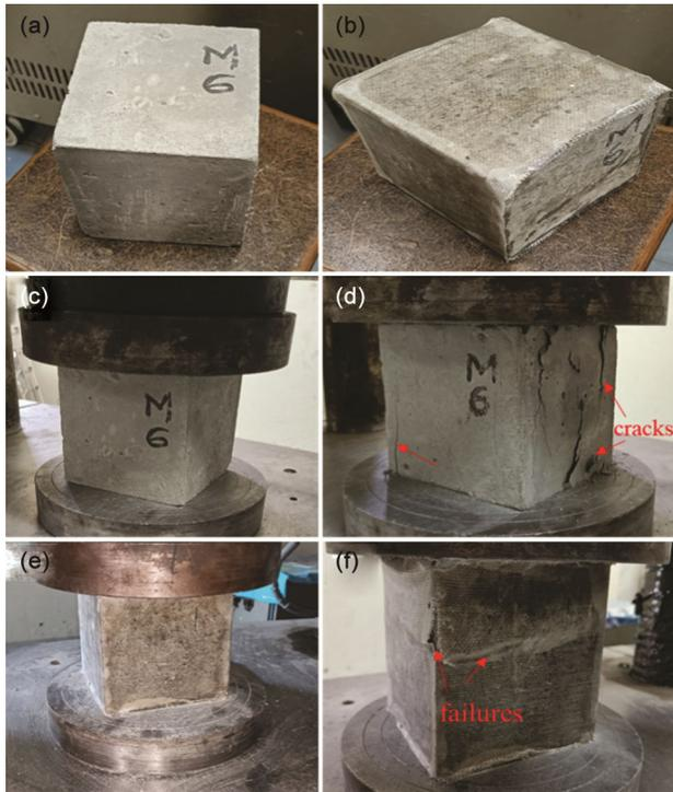
Fig. 2 — Strength testing: (a) Untreated sample (b) FRP treated sample, (c)-(d) untreated sample before and after failure, (e)-(f) FRP treated sample before and after failure due to loading in UTM
