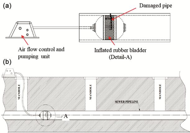
Fig. 4 — Mechanized retrofitting procedure of FRP using inflated rubber bladder technique
