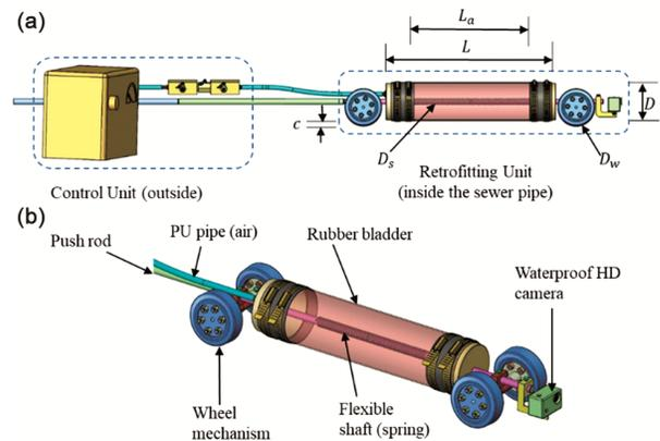
Fig. 6 — Assembly design and parameters of the retrofitting system
