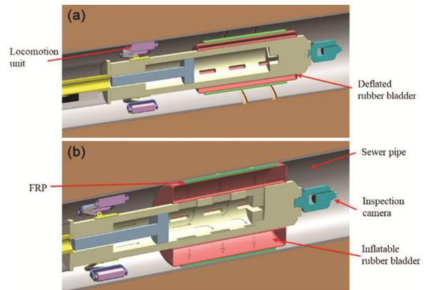
Fig. 5 — Inflated rubber bladder technique with coated epoxy/hardener on GFRP
