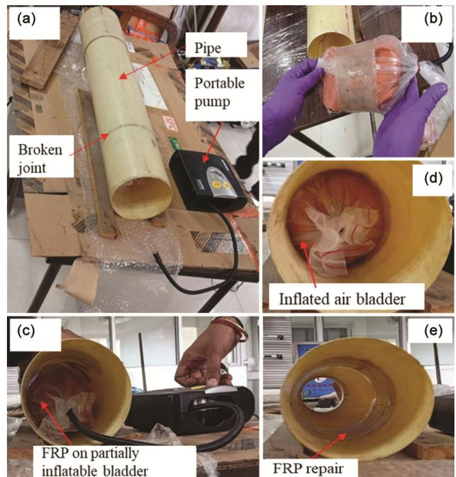
Fig. 9 — Laboratory set-up for FRP repair of internal pipe
