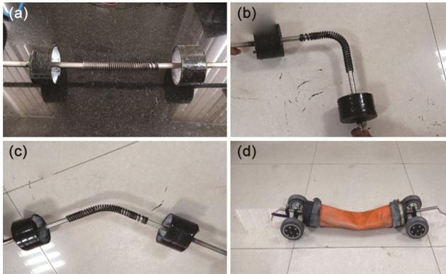
Fig. 7 — Bendable flexible shaft incorporation in retrofit mechanism for better adaptability
