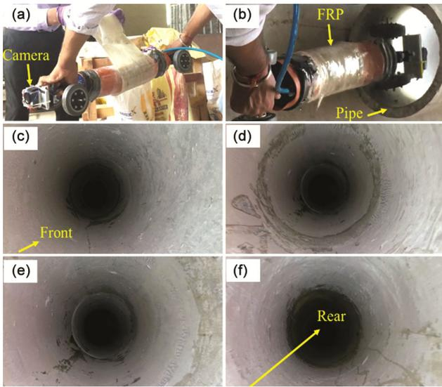
Fig. 10 — Utility of the front mounted HD camera for damage location
