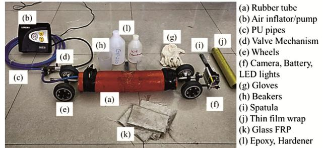
Fig. 8 — The integrated mechanized retrofitting system
