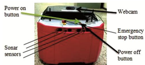
Fig. 3 — Pioneer LX robot and its setup for navigation
