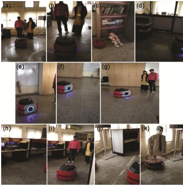
Fig. 6 — The robot guided tour (a) Robot is at its initial state or starting point of the journey and detected the visitors through their faces through the webcam mounted on it. (b) Robot reaches its first visit site, (c) NaO and Amigo Bot are situated at the first visit site of the robot. (d) Robot has arrived at its second visit site, an autonomous car. (e) Robot reached at its third visit site, AMAL. (f) Suddenly robot stops because a visitor is not visible here and waits for the visitor to appear in the camera. (g) Robot sees the visitors and detects their faces and makes an announcement to move. (h) Robot moves towards its next visit site, Tinku a socialistic robot for kids. The robot explains interesting facts about Tinku. (i) Robot moves towards its last journey point (j) Robot arrived at its last visit place; SMART (k) The robot terminates its tour successfully completes its robotic journey.
