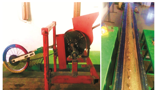
Fig. 4 — Sticky- belt test setup for laboratory evaluations of metering mechanism
