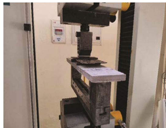
Fig. 2 — Test set up for 4PB
