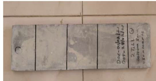
Fig. 1 — Typical specimen for 4PB
