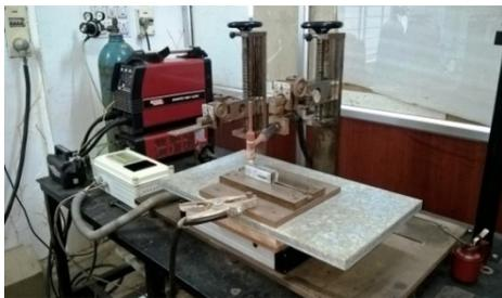
**Figure 1.** GTA heat source setup.
