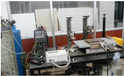
Figure 1. Experimental setup used for surface alloying.
