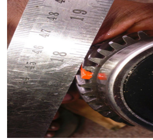
Figure 4. Tooth chipping induced in the gear.
