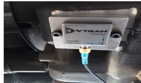
Figure 5. Accelerometer fitted to the bottom of gearbox.
