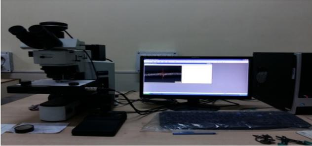
**Figure 3.** Optical microscope (OLYMPUS BX51M).
