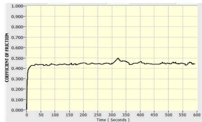
Figure 18. Coefficient of friction vs time for Al-4.5Cu-0.1Cr.
