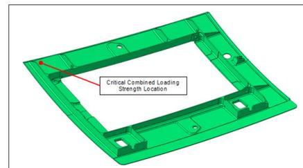
**Figure 16.** Critical limit analysis locations – after latch access door
