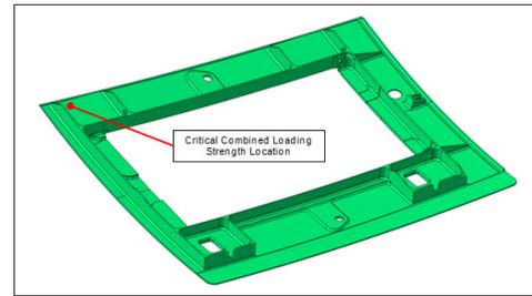
Figure 23. Critical limit analysis locations – after latch access door
