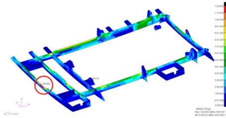
**Figure 26.** Fringe plot of von mises stress – forward latch access door stiffener
