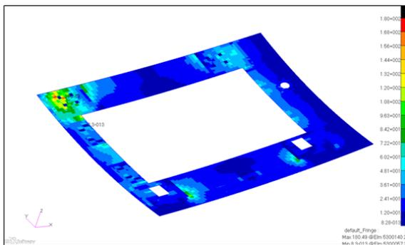
**Figure 18.** fringe plot of von mises stress at Z2 – after latch access door skin
