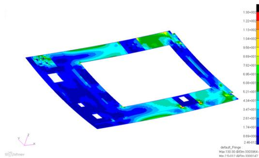
**Figure 12.** Fringe plot of von mises stress at Z1 – forward latch access door skin
