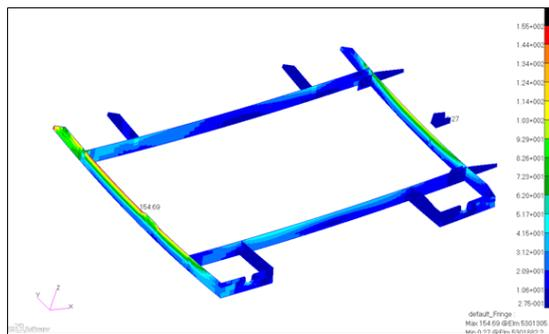
**Figure 20.** Fringe plot of von mises stress at Z2 – after latch access door stiffeners
