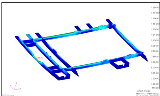
**Figure 14.** Fringe plot of von mises stress at Z1 – forward latch access door stiffeners
