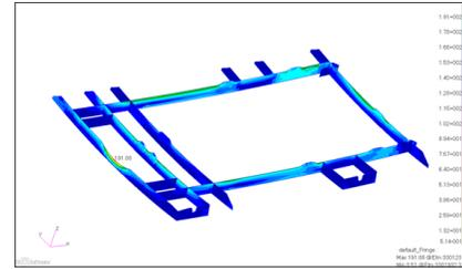
**Figure 15.** Fringe plot of von mises stress at Z2 – forward latch access door stiffeners
