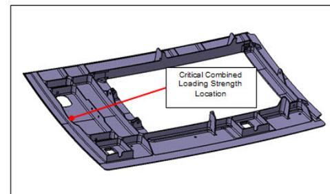
Figure 25. Critical limit analysis locations – forward latch access door
