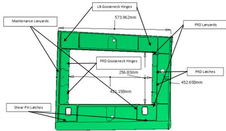
Figure 6. After latch access door
