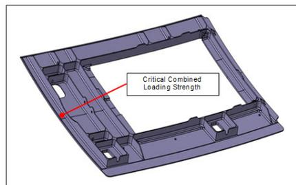
Figure 11. Forward latch access door
