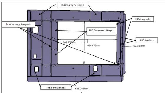
Figure 2. Forward latch access door
