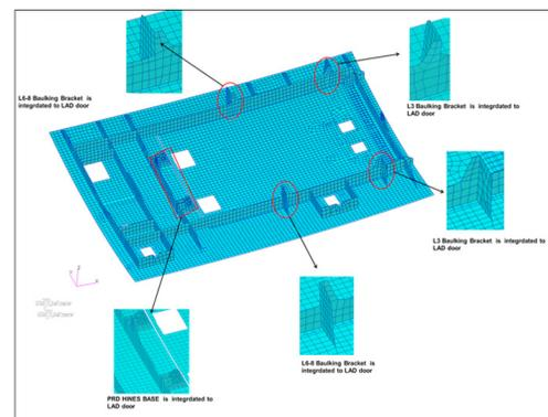
**Figure 21.** Forward latch access door and pressure relief door with casted parts
