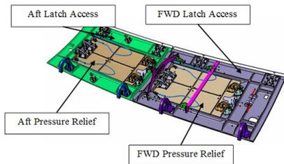
Figure 1. Latch access door assembly
