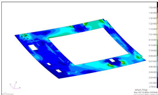
**Figure 13.** Fringe plot of von mises stress at Z2 – forward latch access door skin
