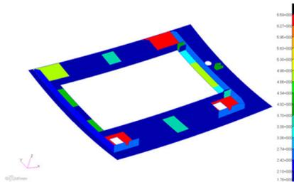
Figure 7. After latch access door thickness plot
