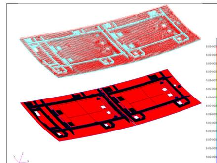
Figure 10. Unit burst pressure load case
