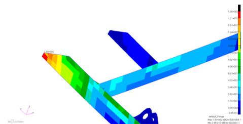
Figure 24. Fringe plot of von mises stress – after latch access door stiffener
