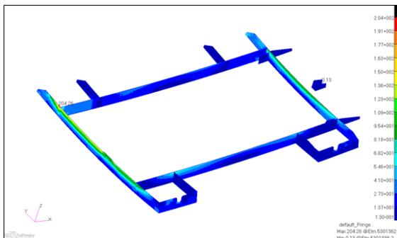
**Figure 19.** Fringe plot of von mises stress at Z1 – after latch access door stiffeners
