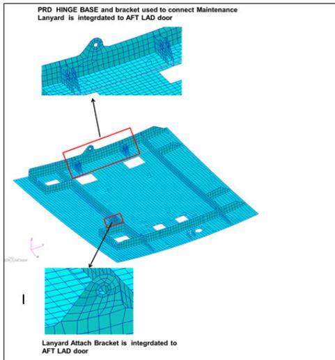
Figure 22. After latch access door and pressure relief door with casted parts
