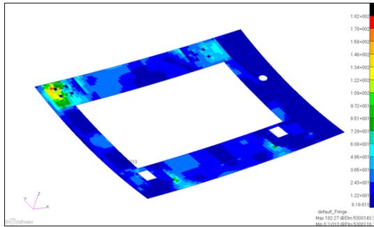
**Figure 17.** fringe plot of von mises stress at Z1 – after latch access door skin
