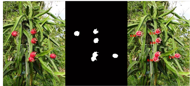
Figure 9. Input, segmented binary image and shape analysis result for dragon fruit.
