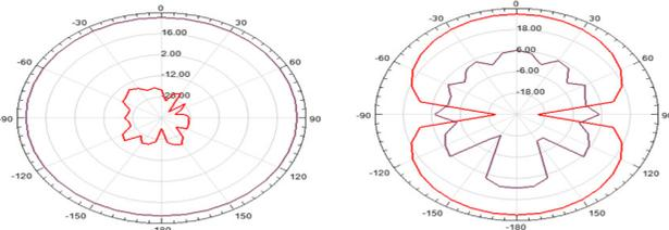
Figure 6. Radiation pattern of filtenna at 15.8 GHz in E and H-plane.
