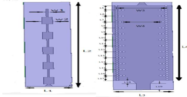
Figure 2. Filtenna model dimensional view.
