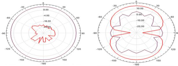
Figure 5. Radiation pattern of filtenna at 14.3 GHz in E and H-plane.
