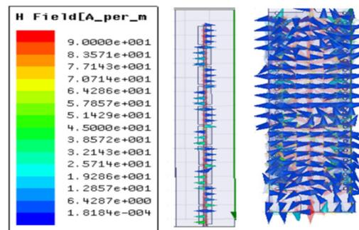
Figure 9. H-field distribution on filtenna at 15.8 GHz.
