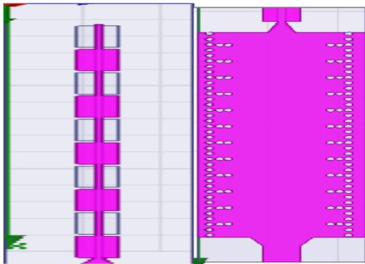
Figure 1. Filtenna model top side view and the bottom side view.
