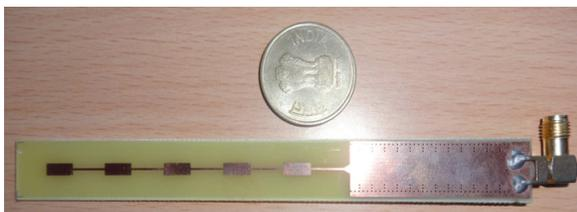
Figure 13. Prototyped filtenna model back view.
