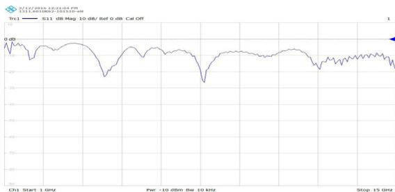
Figure 14. Measured  $S_{11}$  result on ZNB 20 vector network analyzer.
