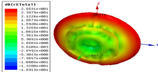
Figure 10. 3-dimensional radiation pattern of the filtenna.
