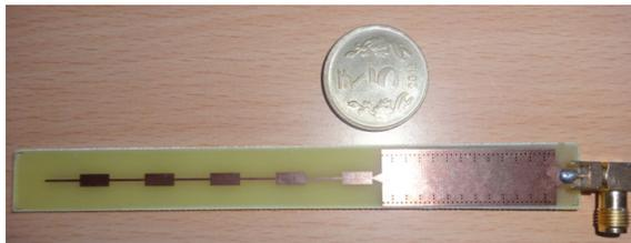
Figure 12. Prototyped filtenna model front view.
