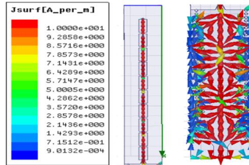
Figure 7. Current distribution at 15.8 GHz.
