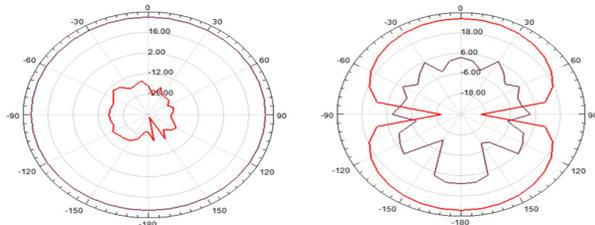
Figure 4. Radiation pattern of filtenna at 12.8 GHz in E and H-plane.
