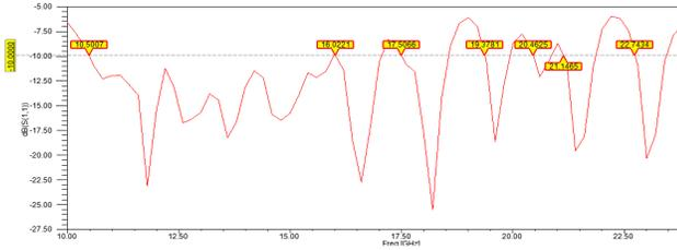
Figure 3. Returnloss vs frequency.
