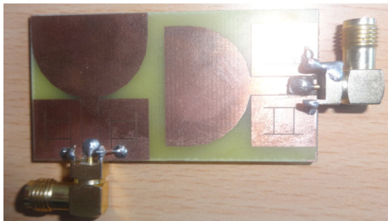
Figure 16. Prototyped Antenna on FR4 Substrate.
