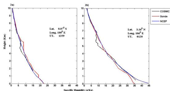
**Figure 2.** Vertical specific humidity profiles measured by COSMIC, nearby radiosonde and provided by NCAR/NCEP reanalysis data on 01 March 2007 at 0120 UTC (left panel, Figure 2a) and 1259 UTC (right panel, Figure 2b).
