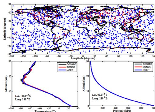
**Figure 1.** Top panel shows global occultations (1465 in number) made by COSMIC satellites (blue circles) and number of radiosonde locations (667 in number) (red circles) on 01 March 2007 and bottom left (right) panel shows vertical temperature (pressure) profile measured by COSMIC, nearby radiosonde and provided by NCAR/NCEP reanalysis data on 01 March 2007. See text for remaining details.
