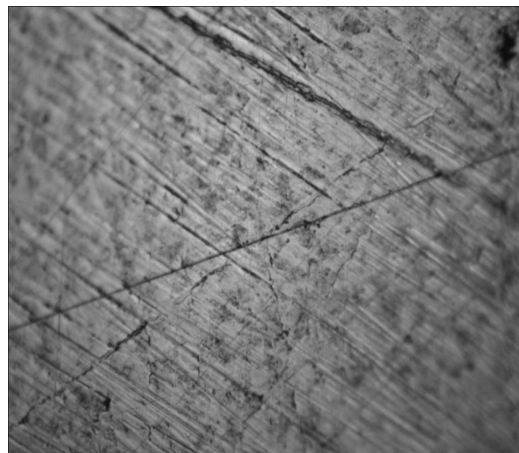
Figure 9. Normalised ferrite-martensite microstructure [500x] at 780°C.
