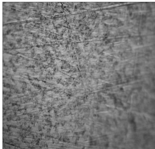
Figure 10. Normalized ferrite-martensite microstructure [500x] at 800°C.
