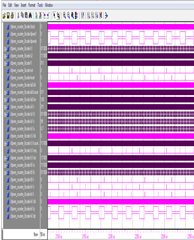
Figure 5. Counter based DPWM generated in Model Sim.
