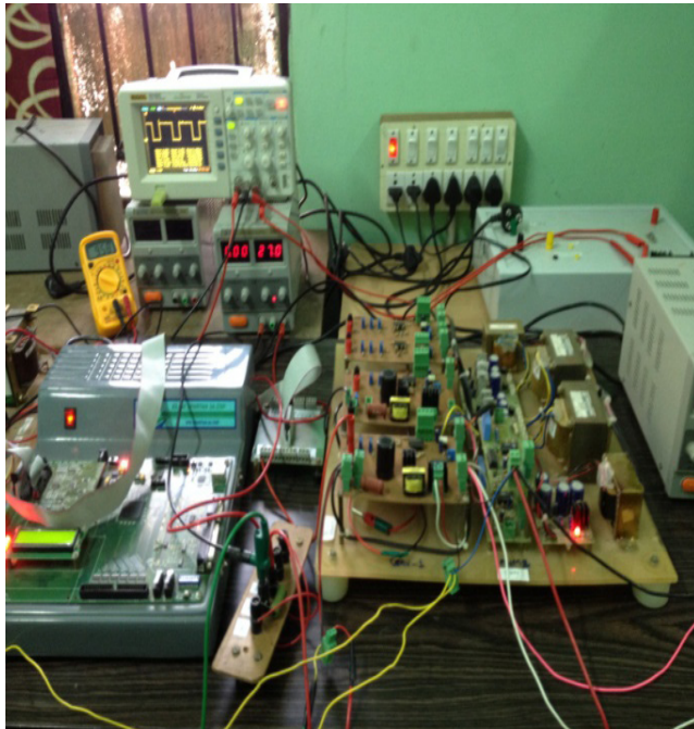
Figure 15. Experimental Setup for the Digital PI based DC-DC Buck Converter.
