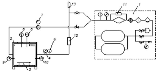
**Figure 2.** Modernized test bench layout: 1 – heat carrier processing system; 2 – experimental model unit; 3 – plate surface, where model liquid is located; 4 – pressure sensors; 5 – temperature sensors; 6 – mobile temperature sensors; 7 – heat carrier flow rate sensors; 8 – gas humidity sensor (hydrometer); 9 – mobile sound frequency and amplitude sensor; 10 – mobile heat carrier flow velocity sensor; 11 – heat-insulated electric heater; 12 – gas analyzer; 13 – utilizer.
