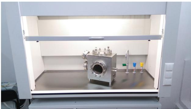
**Figure 1.** Experimental model unit for exploring a model liquid gasification process.
