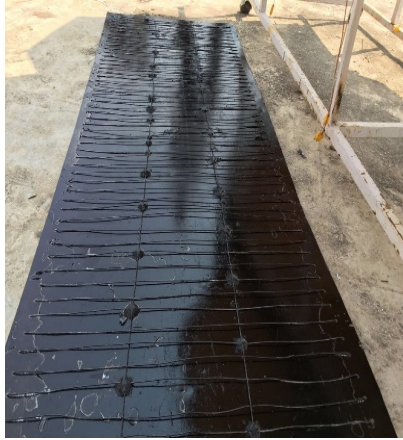
Figure 3b. Wires attached to the flat collector plate.
