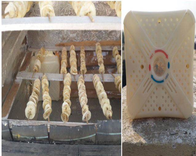
Figure 3c. Dehumidifier inside the drying chamber; Electrical dehumidifier.
