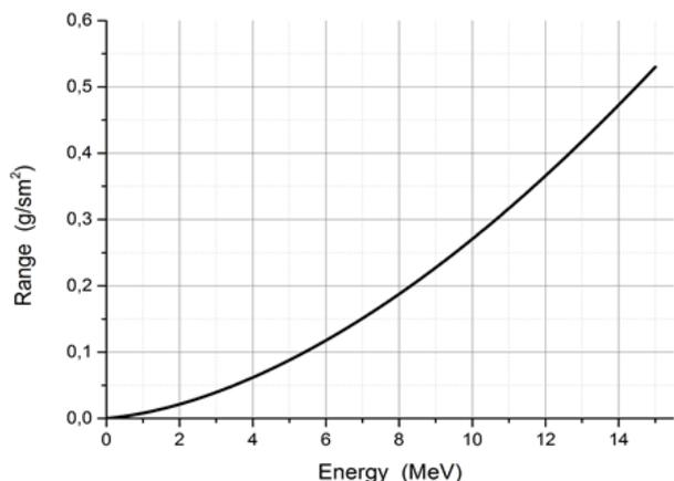
**Figure 1.** Range of protons in metal cadmium.
