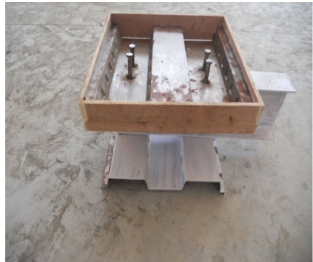
Figure 6. Arrangement of shear connectors and formwork.
