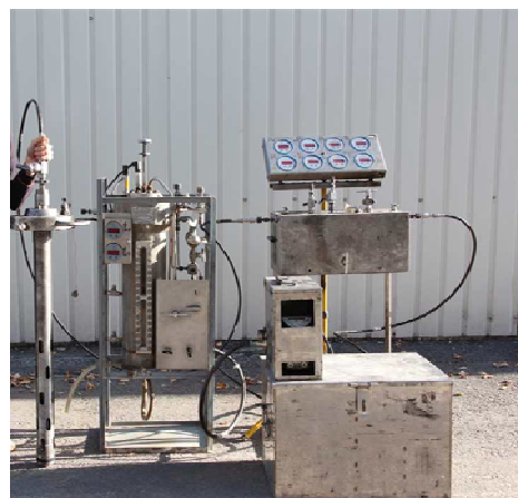
Figure 3. Photo of the multiphase measuring unit produced by TyumenNIIgiprogaz Ltd.
