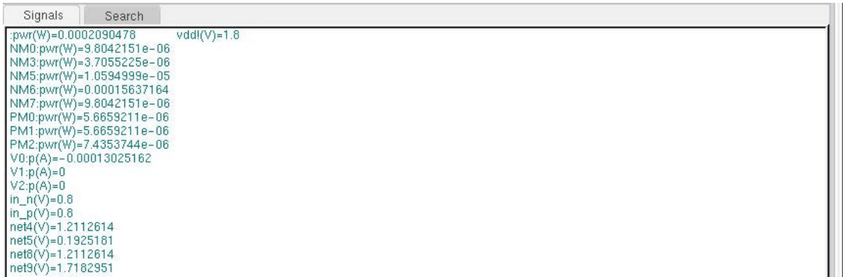
Figure 3. Power observation for conventional op-amp.
