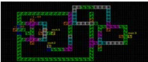
**Figure 14.** QCA layout of RG2.
