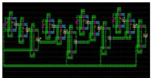
**Figure 18.** QCA layout of novel ripple carry adder..
