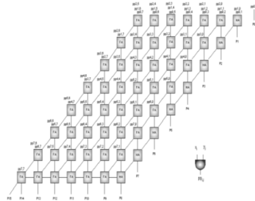
Figure 2. Architecture of array multiplier.
