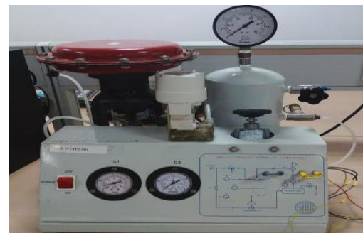
Figure 3. Real-time pressure process station.
