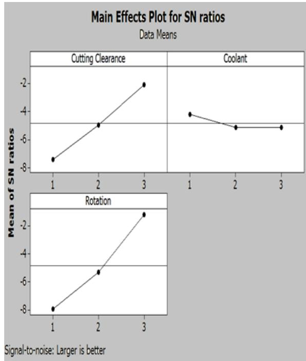
Figure 5. Main effects plot for SN ratios (depth of cut).
