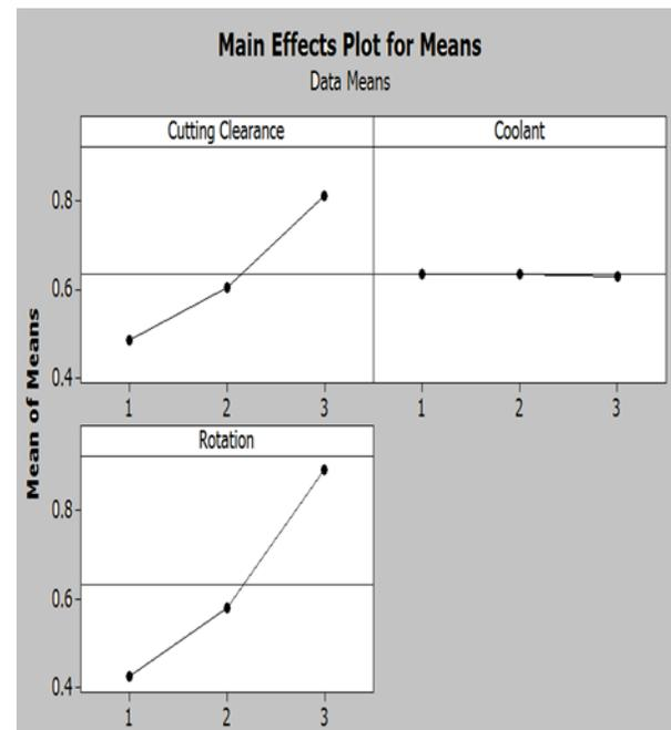
**Figure 4.** Main effects plot for means (depth of cut).
