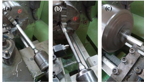
**Figure 1.** Fabrication of the CCM toolpost shaft.
