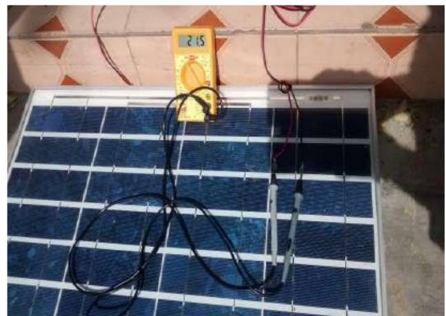
Figure 22. Input voltages from PV panel.
