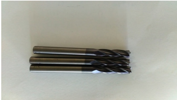
Figure 1. Carbide flat end mill cutter with AlTiN coating.
