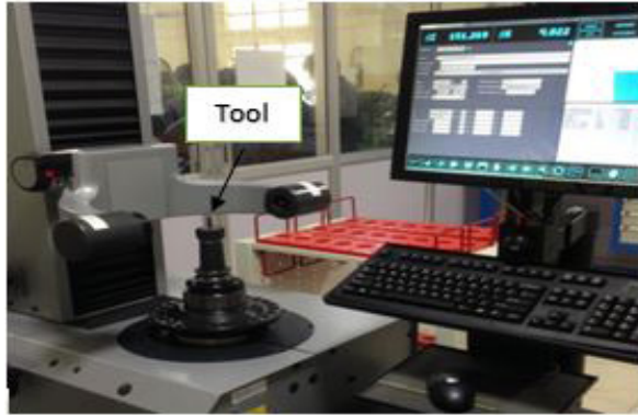
Figure 4. Tool wear measurement in Zoller Presetter.
