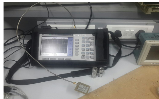
Figure 18. Return loss measured -32.32dB at 2.4302GHz.
