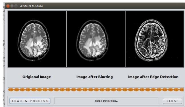
Figure 6. After Applying SOBEL Edge Detection Algorithm.
