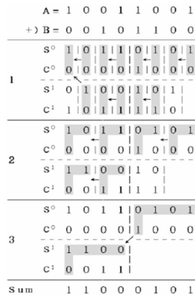
Figure 1. Operation of CSA.
