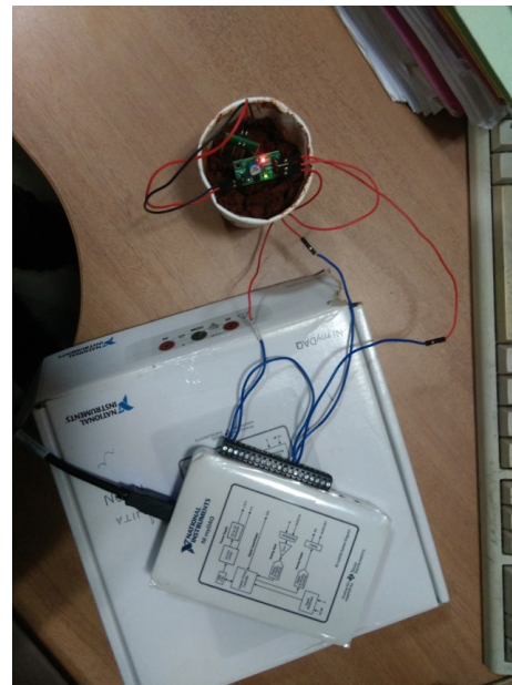
Figure 7. Sensor connected to myDAQ instrument.
